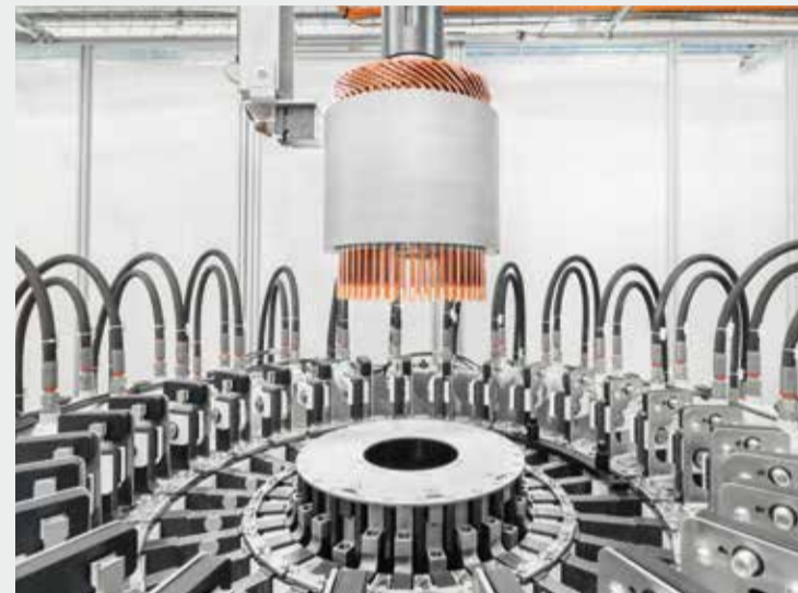
Hairpin production line for the production of stators
